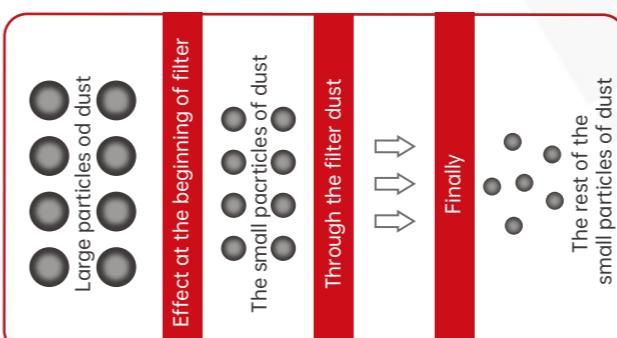
KLC Pre-filter mainly for large particles of dust particles, the main effect at the beginning of a filter for filtering or pre-filtering for effect of filter. Particles of dust particles through the early after small particles remaining effect filter dust. The small particles of dust completely through a filter at the beginning of the end of the effect after the rest of the filter with a little dust.
