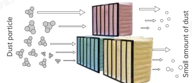
Large particles of dust particles through effective filter was cut at the beginning of the filtering. Since the pre-filter used for large particle size effect filter first, so the small particles of dust will be remained parts through the filter, the pre-filter should be replaced generally three months.
