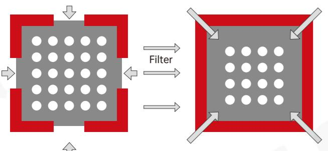
Before filter, gathered different direction and a big number od dust, medium pocket filter is easy, to gather large amounts of dust,due to the bag design, it has laege dust holding capaciy and can hold more dust particles and lock them without overflow
