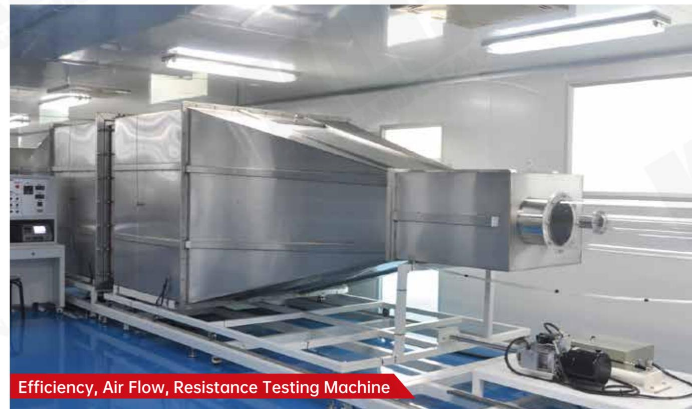
Efficiency, Air Flow, Resistance Testing Machine
